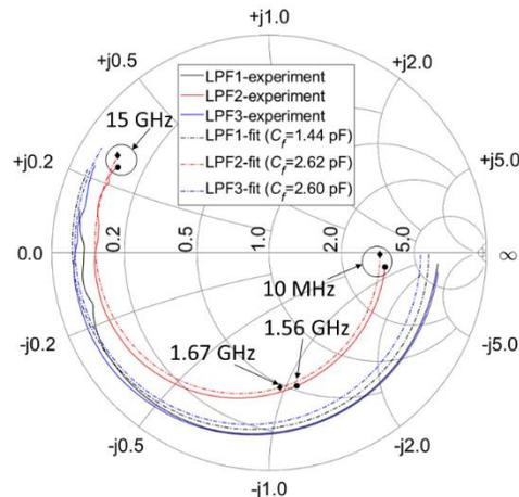
Fig.4: Measured and fitted  $S_{22}$  parameter using the lumped model shown in Fig.1 and the parameters values in Table I for chip no. 3 at 2 V reverse bias
