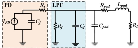
Fig. 1: Schematic of the circuit model for the designed RC low pass filters. Dashed boxes outline the PD and LPF configurations.
