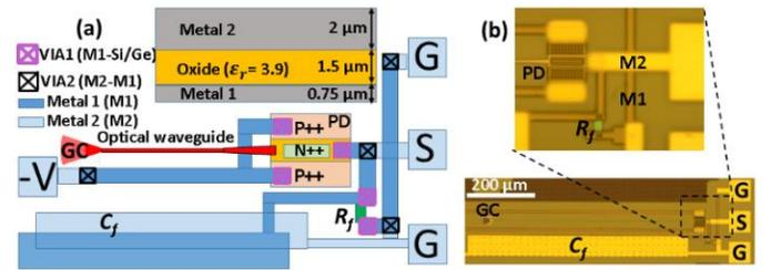
Fig. 2: (a) Cross-section view of the MIM capacitor and layout view of the LPF structure (GC: grating coupler, PD: photodiode, M1: Metal 1, M2: Metal 2) (b) Micrograph of the RC filter structure in an active silicon photonics process.
