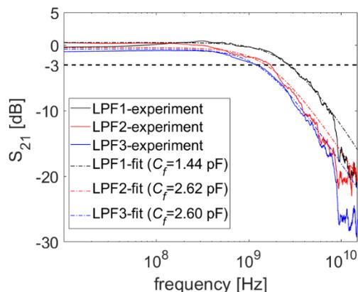
Fig. 3: Measured and fitted  $S_{21}$  parameter using the lumped model shown in Fig.1 and the parameters values in Table I for chip no. 3 at 2 V reverse bias.
